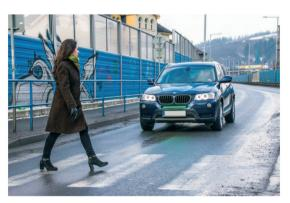
Fig. 4. Vehicle braking information by illuminating the front brake light before a pedestrian crossing
